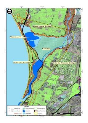
Fig.3 Floodprone areas around the Diep Estuary (based on the 1:100 -year floodline).
