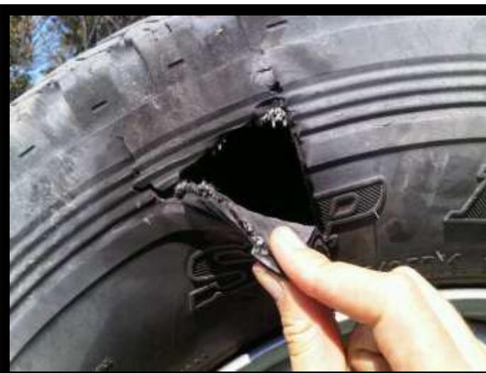
**Figure 18.** Damage to the sidewall of a wheel on the Nissan Patrol fire fighting vehicle.
